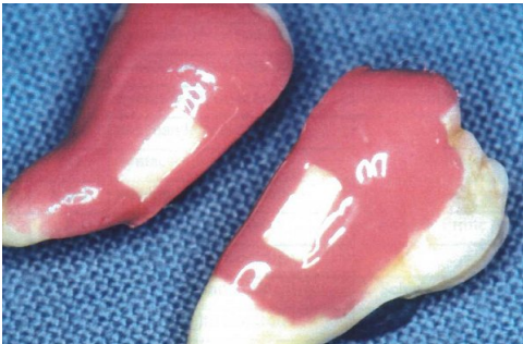
Fig. 1: Specimen coated with an acid resistant nail varnish exposing two rectangular windows.
