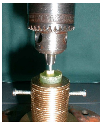
Fig. 6: Fixed tooth in acrylic resin, mounted in the universal testing machine.
