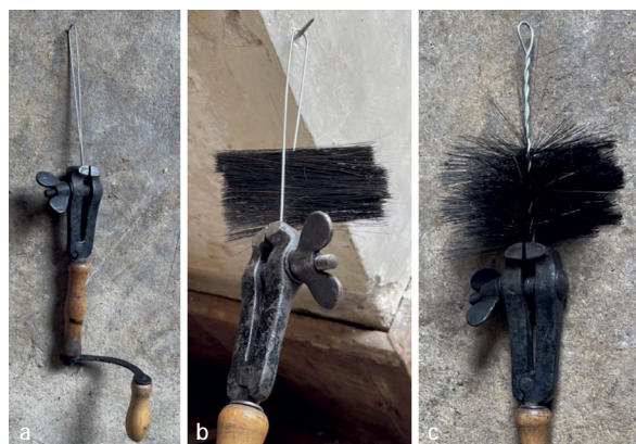
Fig 11 (a)–(c) Hand crank for the manual production of twisted brushes, around 1900. Brush Museum (Todtnau, Germany). Photos: Hans Jörg Staehle.
