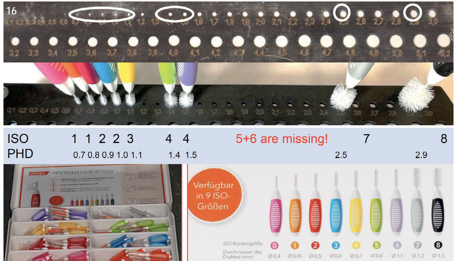
Fig 16 Example of a product system with discontinuous PHD values (here: Elmex, Gaba, Therwil, Switzerland). Top: Measuring plate with different hole diameters corresponding to PHD values. Middle: Measuring plate with equipped IDBs. Sizes 0.7 to 1.0 mm must therefore cover only a single PHD value, size 1.1 mm, however, covers three PHD values, size 1.4 a single PHD value, size 1.5 mm ten PHD values, size 2.5 mm four PHD values, and size 2.9 mm all PHD values from 2.9 mm. Bottom: According to the ISO size information presented in the brochure, the impression of a uniform distribution is created.
