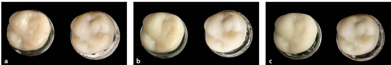
Fig 6 (a to c) Representative images of crowns before (left) and after (right) cyclic loading.
