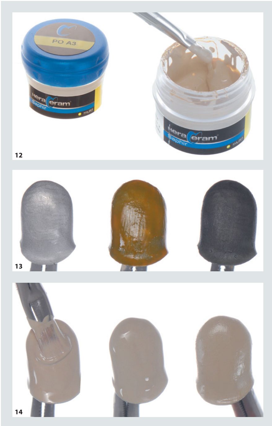
Fig 12 A new generation of paste opaque enables maximum efficiency. Fig 13 The use of HeraCeram NP-Primer makes the oxidation firing unnecessary and prepares the framework surface for the application of the opaque. Fig 14 Thanks to the adhesive force of the newly developed paste opaque, the metal frameworks can be completely masked with a single opaque firing.
