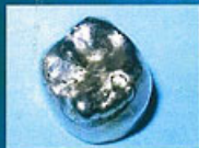
Fig. 4. Filling of the internal absence by welding
