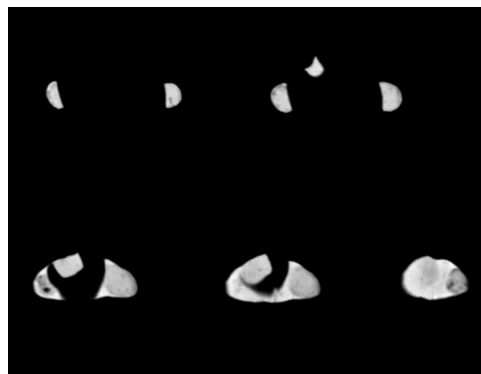
Fig. 2: CT slices of the dental clasp
