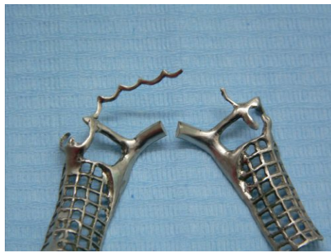
Fig. 2. Fractured continuous clasp and lingual bar.
