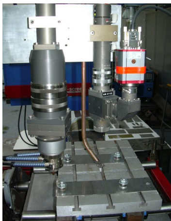
Fig. 6. Welding head of the laser.
