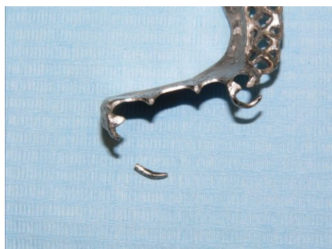
Fig. 4. Broken cast circumferential clasp.
