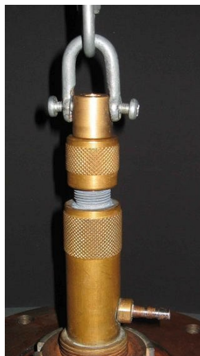
Fig. 7: Experimental apparatus with specimen inside before loading.
