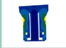
2D-FEM-analysis of micromechanic interface of implant-abutment connection
