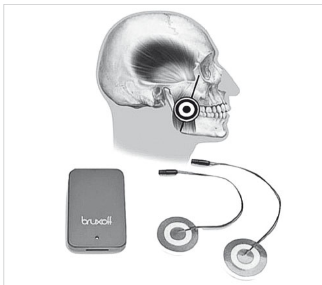
Fig 3 The Bruxoff and the CoDe (Spes Medica) electrode used in this study for the detection of myoelectric signals from the masseter muscles. The concentric ring systems of the CoDe electrodes show higher spatial selectivity with respect to the traditional detection systems and reduce the problem of electrode location, since they are invariant to rotations and reduce EMG cross talk. At the top, a schematic representation of the electrode location over the masseter muscle is shown. Black line: gonial angle-cantus line used as anatomical landmark.
