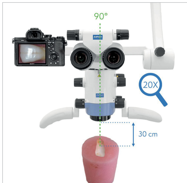
Fig 7 Dental operating microscope setup (vertical positioning) for direct, frontal images.
