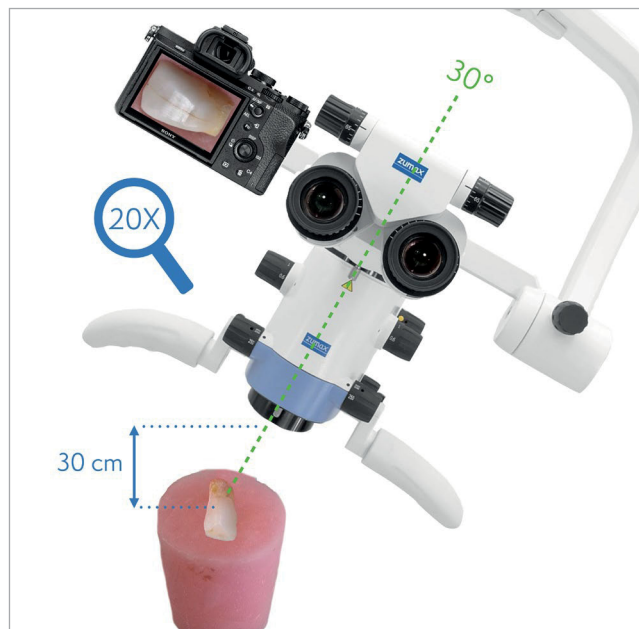
Fig 8 Dental operating microscope setup (30° inclined positioning) for inclined images.
