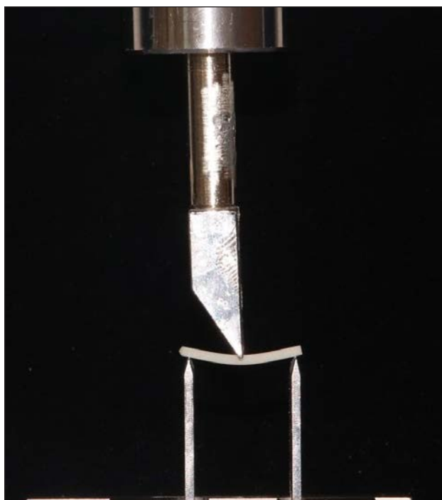
Fig 1 Experimental setup of specimens to measure flexural strength.
