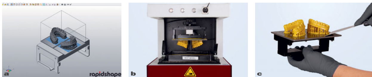
Fig 7 (a) Software preparation for the AM process that allows for the positioning of the objects on the building platform, and adding the corresponding supportive material for its fabrication, (b) 3D polymer printer (RapidShape D30) used for manufacturing the casts, and (c) printed diagnostic casts on the building platform immediately after manufacturing.
