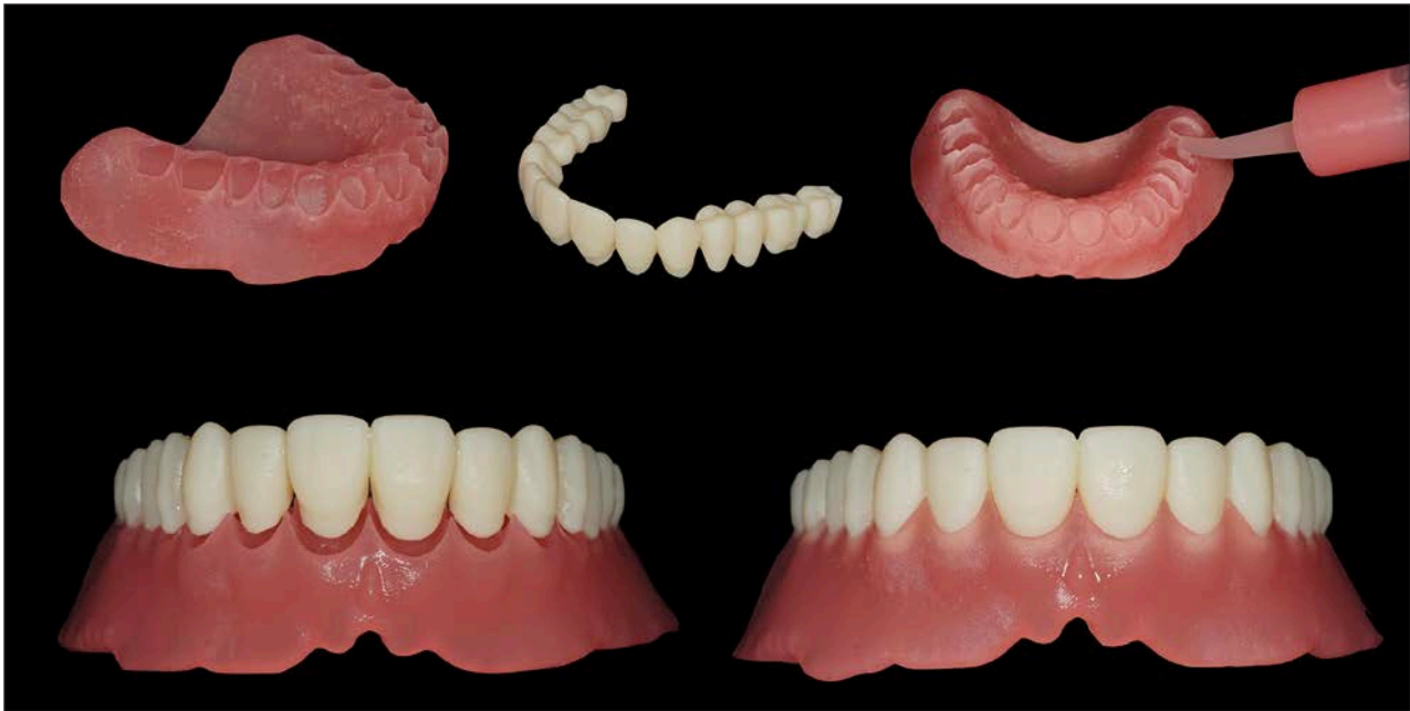
Fig 1 Printed denture base and teeth with assembly process using DLP printing technology.
