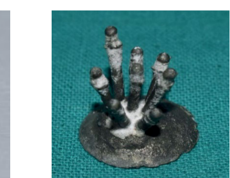
Attachments after casting
