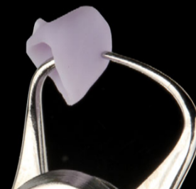
Fig. 10 - Crown after milling with 1.6 mm thickness
