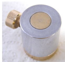
Fig. 3: Holder for adjusting the veneering thickness
