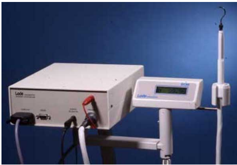
Abb. 3: ECM III, an electric conductive measurement device from Lode Diagnostics, Groningen, The Netherlands
