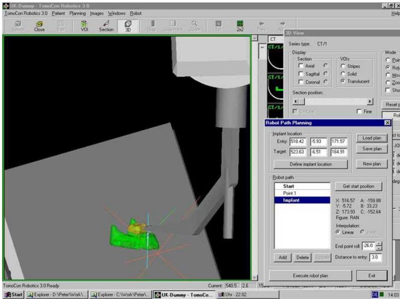
Controlling the plan before drilling
