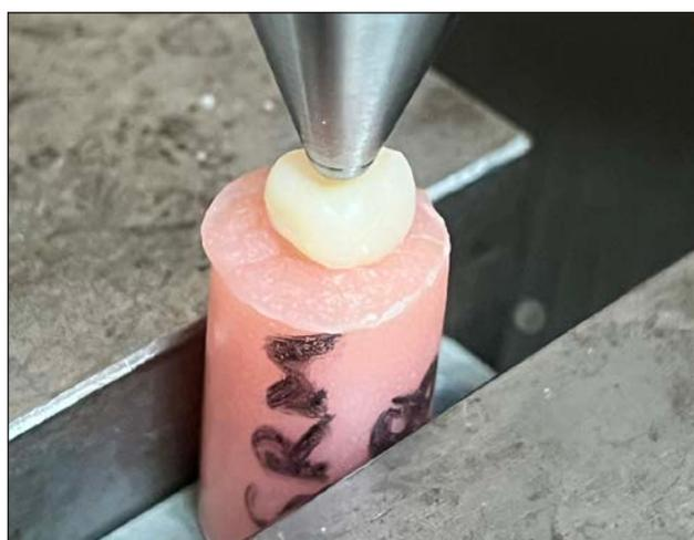
**Fig 2** Fracture resistance test.
