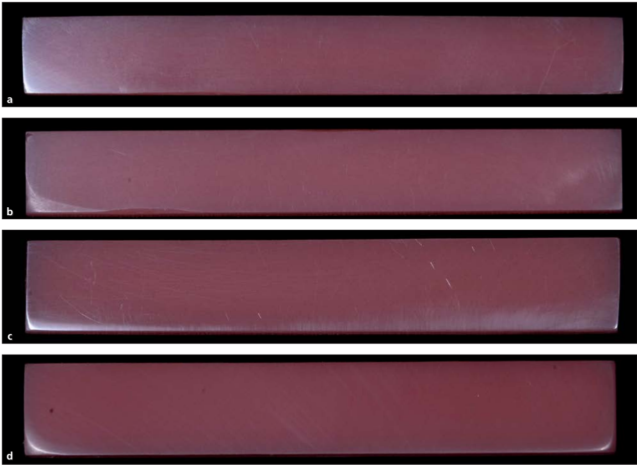
Fig 3 Samples were made of each resin manufacturing type according to the established measurements: (a) conventional, (b) microwave-processed, (c) milled, and (d) 3D-printed.
