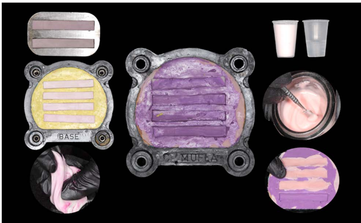
Fig 2 All materials used for the confection of conventional and microwave-processed samples, including the mold and muffle used.
