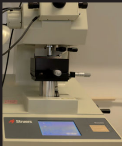
Figure 5 – Microhardness Indentation Machine ( Duramin ) Knoop Diamond Indenter. 98.12 mN load 30 seconds. 12 measurements in each specimen
