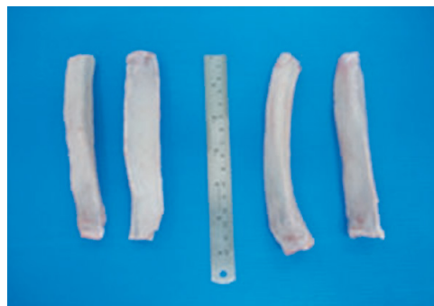
Fig. 2: Sections of fresh rib bones from adult pigs were selectively demineralized by timed immersion in 1 % EDTA.
