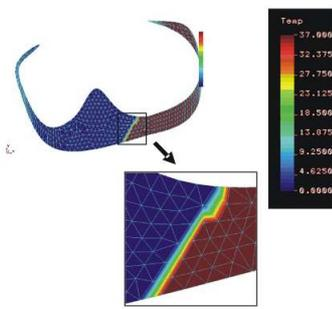
Fig. 3. Temperature distribution for the Akers clasp in case of thermal variations from 37°C to 0°C.
