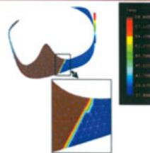
Fig. 4. Temperature distribution for the back action clasp in case of thermal variations from 37°C to 60°C.
