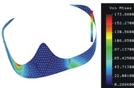
Fig. 1. Von Misses equivalent stress resulting the simulation of a static charge (average force of 20N) in the Akers clasp.
