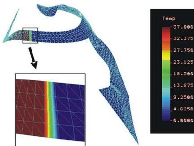
Fig. 5. Temperature distribution for the back action clasp in case of thermal variations from 37°C to 0°C.
