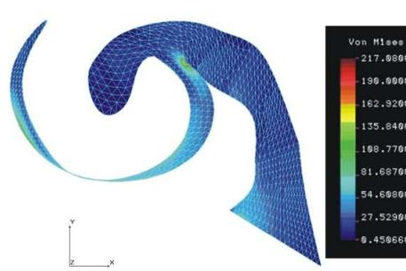
Fig. 2. Von Misses equivalent stress resulting the simulation of a static charge (average force of 20N) in the back action clasp.
