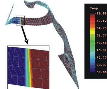
Fig. 6. Temperature distribution for the back action clasp in case of thermal variations from 37°C to 60°C.
