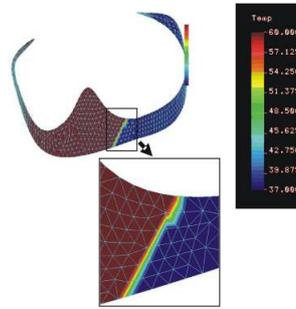
Fig. 4. Temperature distribution for the back action clasp in case of thermal variations from 37°C to 60°C.
