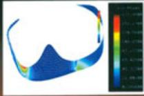
Fig. 1. Von Mises equivalent stress resulting the simulation of a static charge (average force of 20N) in the Akers clasp.
