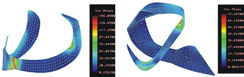
Fig. 7. Equivalent stress distribution when static (20N) and thermal charges (0°C) were cumulated:
