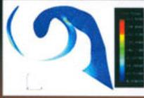
Fig. 2. Von Mises equivalent stress resulting the simulation of a static charge (average force of 20N) in the back action clasp.
