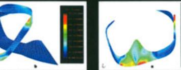
Fig. 8. Equivalent stress and displacement distribution when static (20N) and thermal (60°C) charges were cumulated. a. Akers clasp, b. back action clasp.
