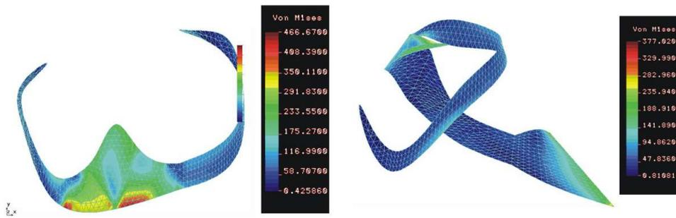
Fig. 8. Equivalent stress and displacement distribution when static (20N) and thermal (60°C) charges were cumulated: a) Akers clasp. b) back action clasp.
