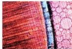
Fig. 3: Unbrushed control specimen, the dentin adhesive layer is visible. Polarized light, 64x.
