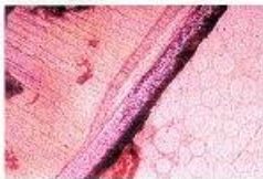
Fig. 4: Brushed specimen, Prime & Bond NT, 800 cycles. Polarized light, 64x.
