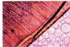
Fig. 5: Brushed specimen, Optibond Solo, 800 cycles. Polarized light, 64x.
