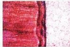
Fig. 6: Brushed specimen, Prime & Bond NT, 1600 cycles. Polarized light, 64x.
