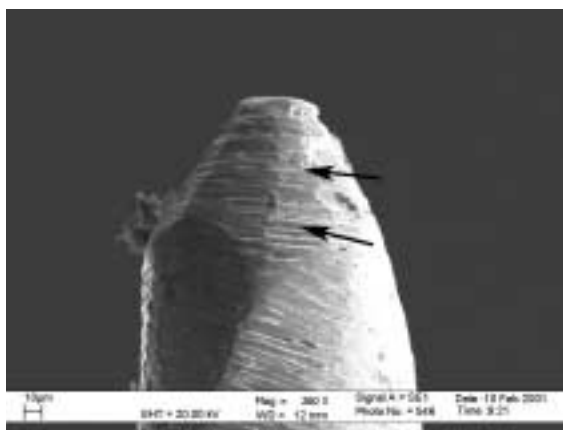
Fig 4 Presence of metallurgic defects (micro-cracks, machining marks and metal flash) on the surface of a new NiTi instrument (indicated by arrows).
