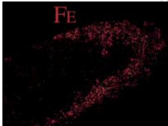
Fig 10 Presence of Fe deposits on the tip of a NiTi instrument after NaOCl treatment.
