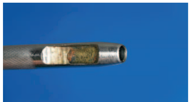
Fig 2 The punch to make the facial opening.
