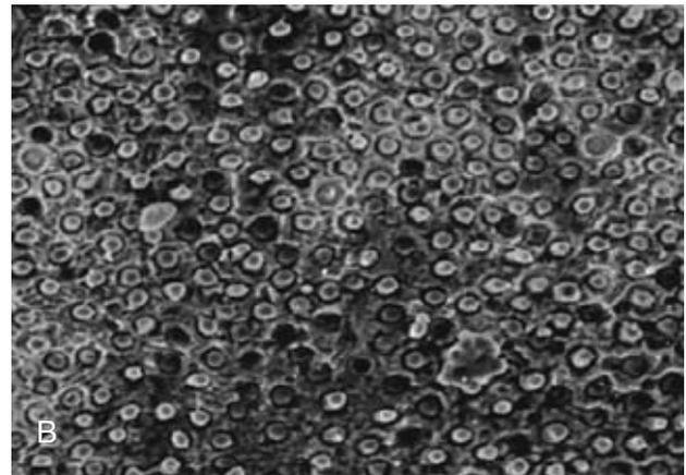
**Fig 2** SEM observations of the fractured surface along the dentine side of one specimen. (A) Mixed failure is observed. Most of the surface is covered by an adhesive layer although some dentine is exposed. (B) At a higher magnification of the exposed dentine, resin tags in the tubule entrances are observed.
