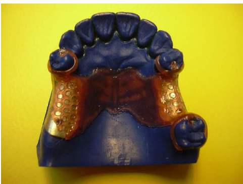
Fig. 5. After light-curing the wax pattern "Ti Light" turns his colour from pink to yellow,
