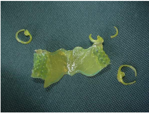
Fig. 10. Cracks at both materials
