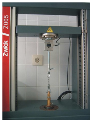
Fig. 2: Special designed apparatus mounted in a universal testing machine.
