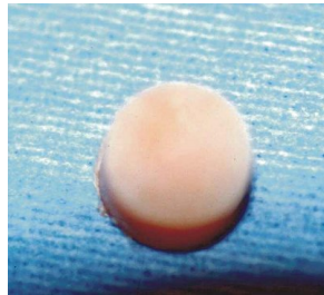
Fig. 5: Prepared specimen (diameter: 8 mm): thickness of 4.0 mm ( \pm 0.5 mm) and a cortical layer of 1.5 mm ( \pm 0.2 mm).
