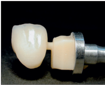
Figs 11 and 12 View of the crown directly after the milling process.
