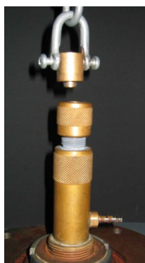
Fig. 5: Experimental device after loading until fracture.
