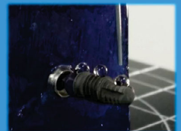
Figure 3- Analysis of wettability with deposition of sessile drop in 3 different locations on the implants surface (Vellox®)
