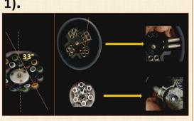
THE G-FORCE AT 2700 RPM IS CLEARLY IN EXCESS OF THE 400g RECOMMENDED IN THE LITERATURE¹ (Table 2). ONE SIZE CLEARLY DOESN'T FIT ALL, PLUS AN UNKNOWN FACT THAT THE RPM CAN BE ADJUSTED TO THE G-FORCE REQUIRED<sup>2</sup> AS PER THE FORMULA G FORCE= 1.12 X CENTRE-OF-CENTRIFUGE TO TUBE DISTANCE X (RPM/1000)<sup>2</sup>
