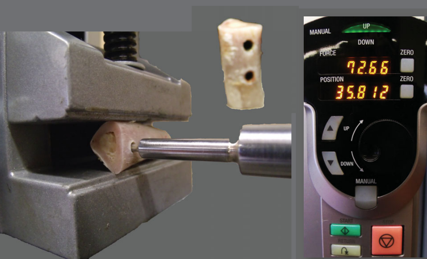
Removal torque test performed in a universal testing machine with a speed of 1.96 mm / min.
