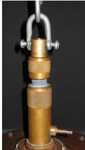
Fig. 6: Experimental apparatus with specimen inside before loading.
