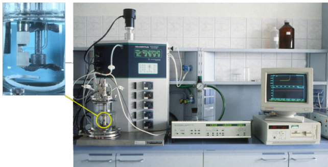
Fig. 1: Test system with bioreactor and potentiostat; electrochemical measuring rod is shown in enlargement
