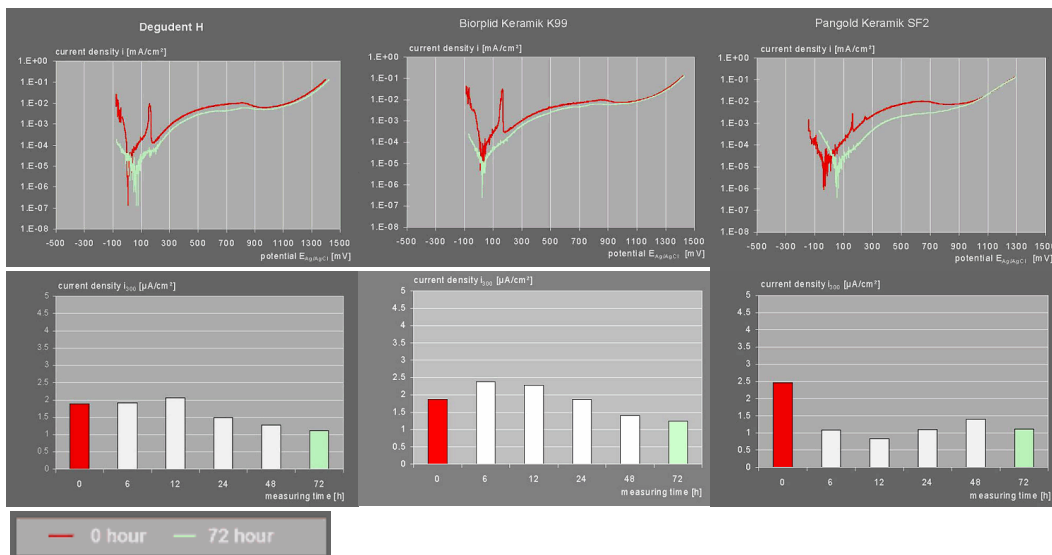
Fig. 5: Long-term behaviour of test materials in dextrose food solution after different times
