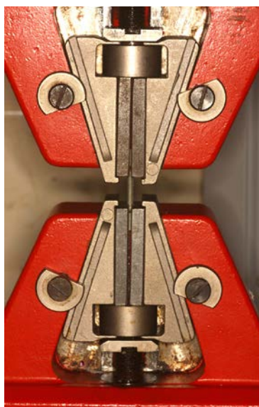
Fig 2 Tensile test in progress.
