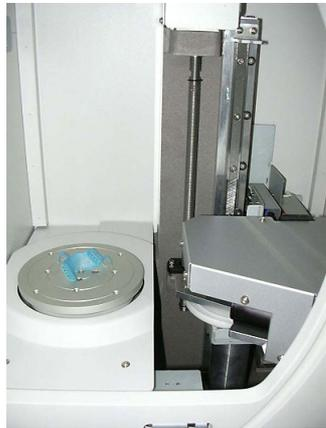
Fig. 3a and 3b: Scanning the Wax-pattern - reverse engineering method
