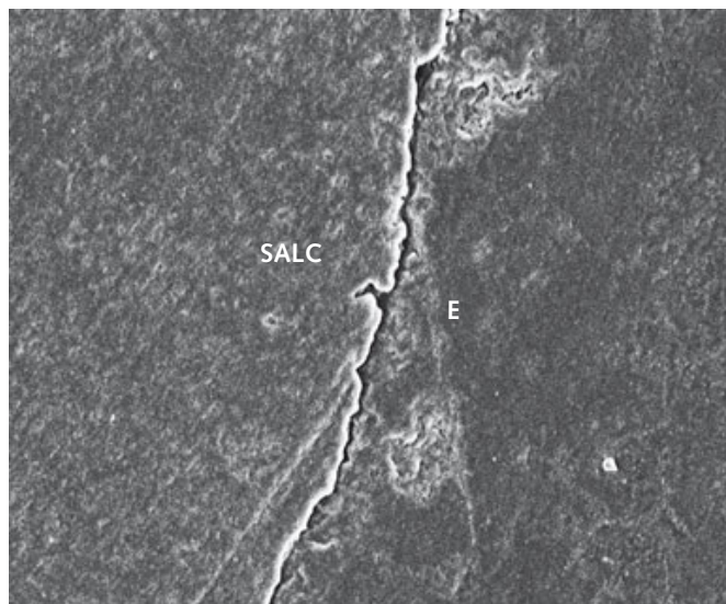
Fig 3 SEM image of a gp formation between self-adhesive resin cement (Maxcem Elite, Kerr, CA, USA) and the enamel margin of a ceramic inlay (300x) (SALC: self-adhesive luting composite; E: enamel).
