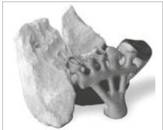
**Fig. 18-39 Casting upon devesting** Note the smooth, matte surface of the casting and its reproduction in the investment. Picture courtesy of PxDental Corp.
