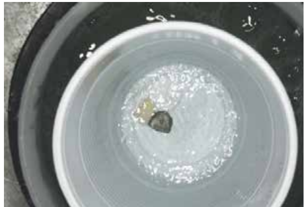
Fig 6-17 ...and the RBFDP can then be cleaned of more firmly adhering blasting media residues in the ultrasonic bath with 99% isopropanol.
