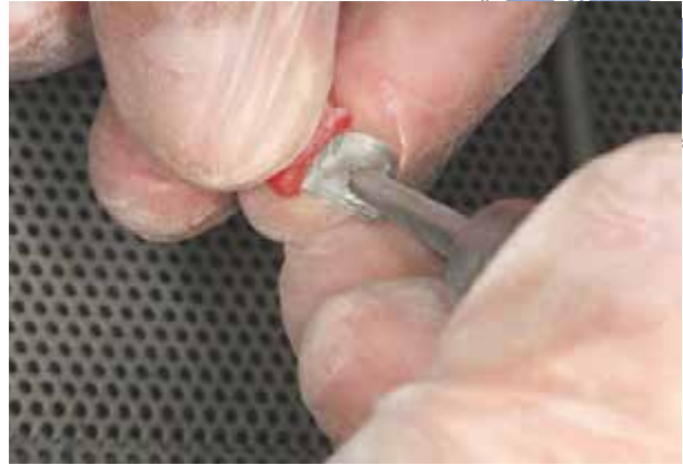
Fig 6-15 The retainer wing is air abraded with 50 µm alumina particles at 2.5 bar pressure in order to achieve a roughening, cleaning, and activation of the bonding surface. The uniform matting of the metal surface can control the effectiveness of the air abrasion process.
