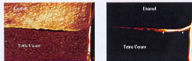
Fig. 3: CLSM image in reflection (left) and reflection (right) mode from a specimen of group J. A dye penetration (arrows) between restorative material and enamel occurred (here grade 1).
