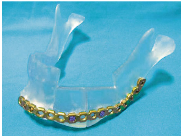
Fig 8 Three-dimensional printed mandibular cast and pre-bending of the reconstruction titanium plate to produce a customised reconstruction titanium plate.
