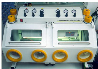
Fig. 3: special sand-blast-blower "Multipoint 2000"
