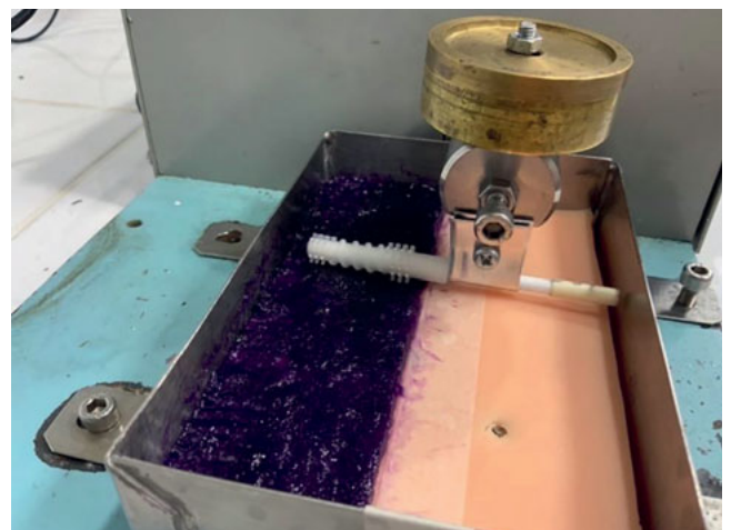
Fig 3 The silicone head was attached to a V.P.2000 toothbrushing machine.
