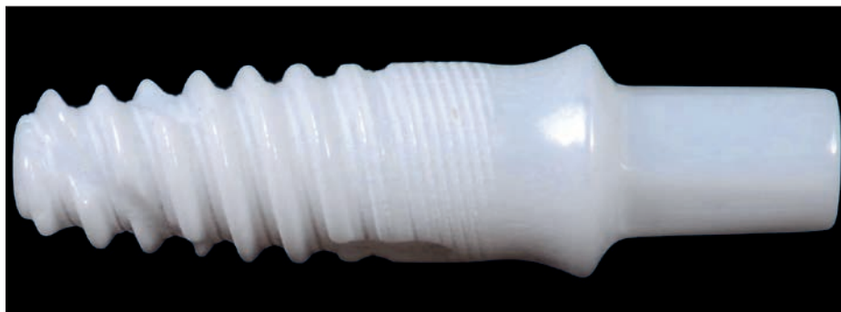
Fig 4 Experimental one-piece 3D-printed zirconia implant. The substructure was 3D printed with an ACJ ceramic 3D printer (PGJ180; Thales Medtech) using a 3Y-TZP ceramic nanoparticle suspension.
