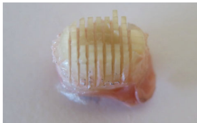
Fig 1 Composite-dentin sticks attached to the underlying composite resin surface. Sticky-wax is placed under the composite resin, so that specimens can be mounted on a chewing simulator plate.
