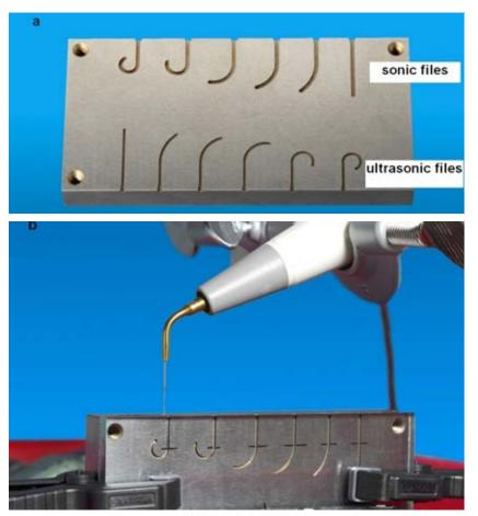
**Figure 6a–b** Figure 6 shows the obtained artificial steel root canal model for the testing of sonic files (**a**, 1.2 mm diameter, upper row) and ultrasonic files (**a**, 0.8 mm diameter, lower row). The cyclic fatigue testing took place with the Tiratest 2720 at 120 mm/ min (**b**). The starting point was placed at the canal orifice at 9 mm (**b**, marked line). The file penetrated 10 mm into the canal and stopped 1 mm before reaching the apex to ensure the working length (19 mm).
