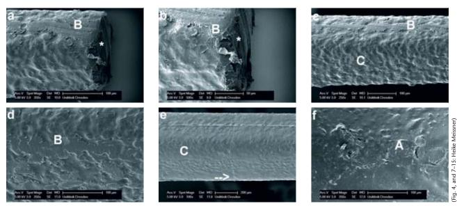
**Figure 15a–f** EndoActivator-tip showing no signs of fracture but crack initiation at the periphery of the instrument (**e**; arrow). Although, surface wear (**f**; A) and a levelled surface relief (**a–d**; B) with erosion of the instrument tip and crack initiation at the periphery of the instrument are visible (**e**; arrow).
