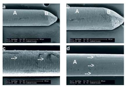
**Figure 11a–d** ESI-tip showing no signs of fracture or crack initiation at the periphery of the instrument. Although, low surface wear (**a**, **b**, **d**; A) and a levelled surface relief (**a–b**; B) with scratches, material abrasion (**c**; arrow) and erosion of the instrument tip are visible (**a–b**; B).
