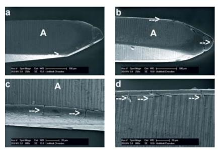
**Figure 9a–d** Irri S tip showing signs of crack initiation at the periphery of the instrument without the fracture of the tip (**a–d**; arrow). Presence of manufacturer dependent material characteristics on the surface of the instrument (A).
