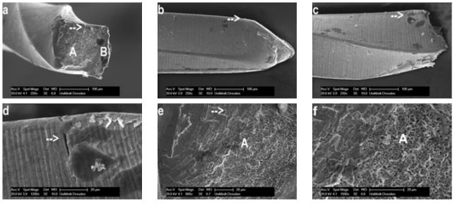
Figure 8a-f Fracture surface of an Irri S tip (a, e, f) showing fatigue striations, crack initiations (arrows) and areas not involved in fatique striations (a; B). The profile of the tip reveals the presence of further crack initiations at the periphery of the instrument (b, c, d; arrows). Note the areas with skewed dimples on high power view (f; A).
