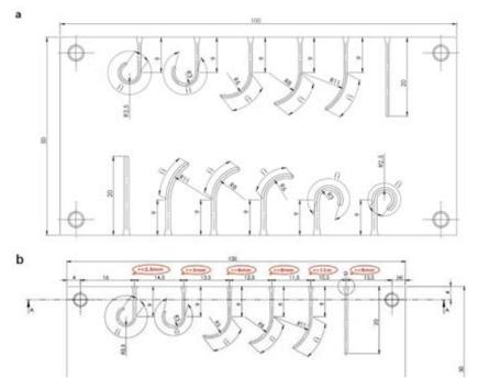
**Figure 5a–b** Design drawing of the root canal model. With the results of the diameter and radius of curvature measurements, a root canal model was obtained (a-b). The arc length of the artificial root canals was always defined at 20 mm, the root canal diameter at 0.8 mm for ultrasonic files (b) and 1.2 mm for sonic files (a; lower row).
