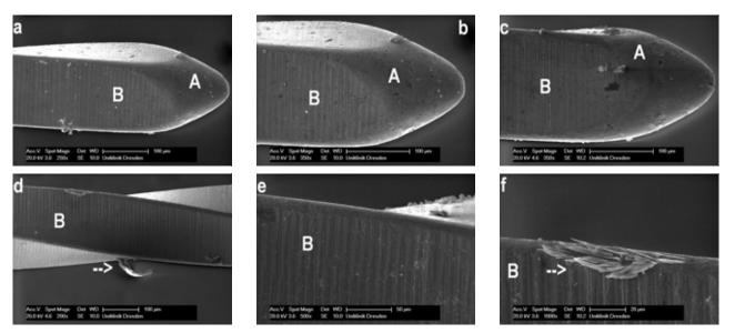
Figure 7a-f Initial state of the Irri S instrument tip: Instrument surface showing no surface wear (a-c; A) but manufacturer-dependent material characteristics (a-f; B). In addition, fanned out areas were detected at the material surface (d, f; arrow).
