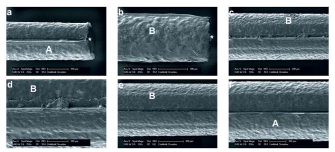
Figure 14a–f Initial state of the EndoActivator-instrument tip: Instrument surface showing no surface wear (a, f; A) but manufacturerdependent material characteristics like the blunt tip (a–b; \*) and polymer structure adhesion at the synthetic joint (a, c–f).
