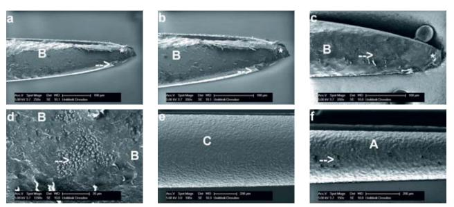
**Figure 13a–f** Eddy tip showing no signs of fracture or crack initiation at the periphery of the instrument. Although, surface wear (**a–d**, **f**; A) and a levelled surface relief (**a–d**; B) with scratches (**a–b**, **f**; arrow), material abrasion (**c**, **d**; arrow) and strong erosion of the instrument tip are visible (**a–c**; \*).
