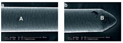
**Figure 10a–b** Initial state of the ESI-instrument tip: Instrument surface showing no surface wear (**a**; A) but manufacturer-dependent material characteristics (**b**; B).
